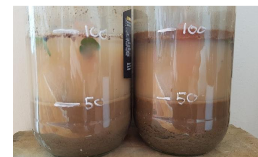
Figure 3: Soil Test Results - Front yard (left), Rear yard (right) Jars calibrated for volume
